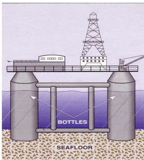
Figure 4. A bottle-type submersible
